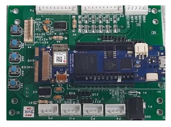
The Arduino Vidor 4000 is used to build this PWM Controller, which consists of one Cortex M0+ Microcontroller and Intel Cyclone10 FPGA.
