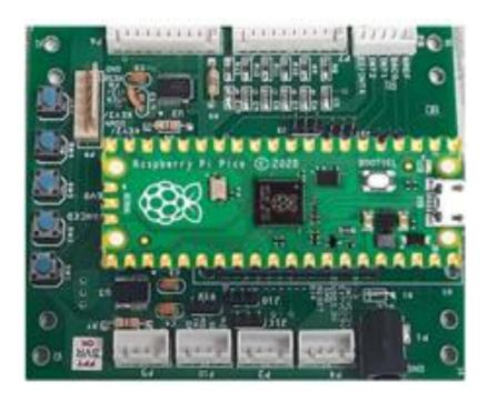
The **RP2040 Dual Core** Processor is used to build this PWM Controller, which consists of Dual Core Cortex M0+ Microcontroller with Flash Ram, PWM, ADC and many on board features.
