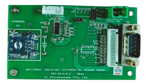
A Signal Conditioner Board for QEP or Proximity Sensor for speed measurement of Motor.
